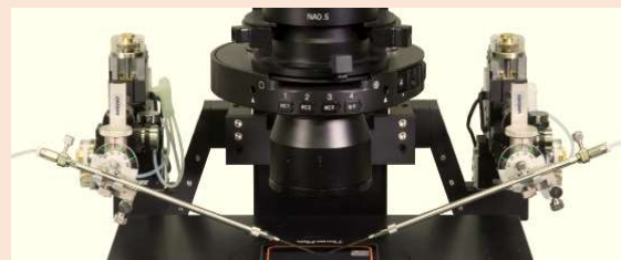
Pipette angle 15 degrees
